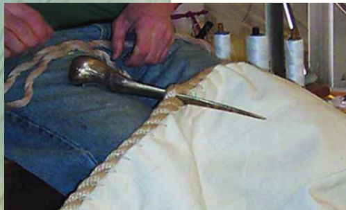
Using a Swedish fid to attach a leech cringle to the Nina's forecourse.
